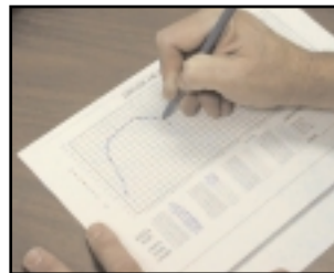
Step 4: Connect points to determine temperature curve. Map the dryer in the morning and in the evening to account for changes in the environment.
